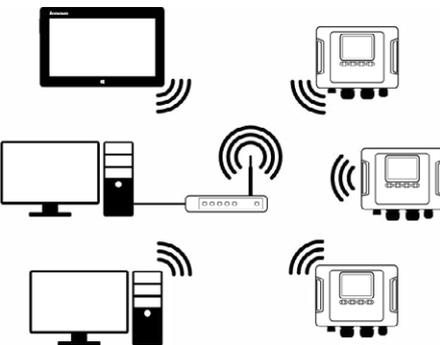
PQM-710 and PQM-711 have a **built-in GPS receiver** ensuring real time clock accuracy and an integrated **GSM modem** that facilitates remote analyzer operation. Furthermore, PQM-711 is also equipped with a **transient recorder** (sampling frequency 10 MHz, voltage range **up to  $\pm 8000$  V**).
